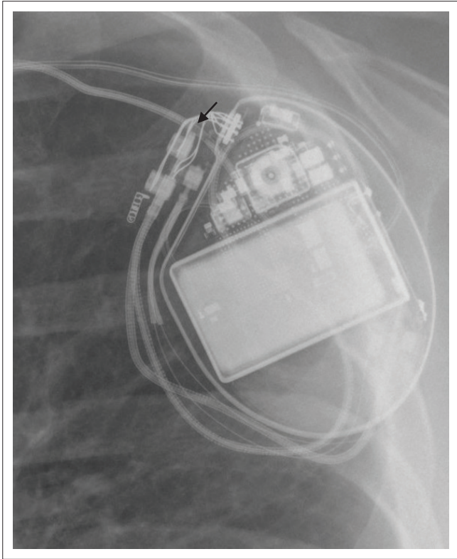
FIGURE 9: A dual-lead implantable cardioverter defibrillator with a subtle fracture (arrow) in the proximal portion of the right atrial lead, close to the generator.
